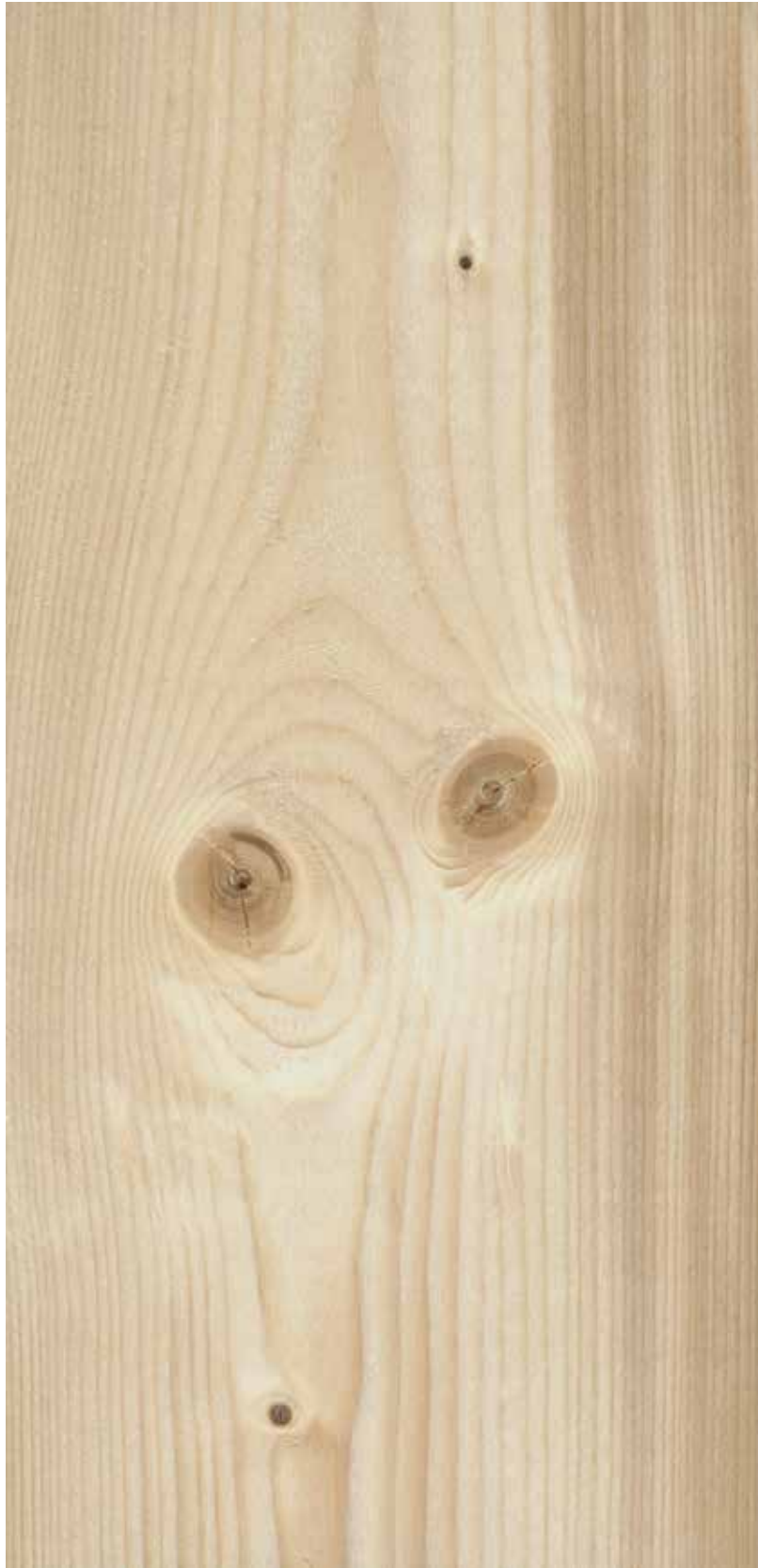
Figur 13. Mye brent. Planken vrakes.
