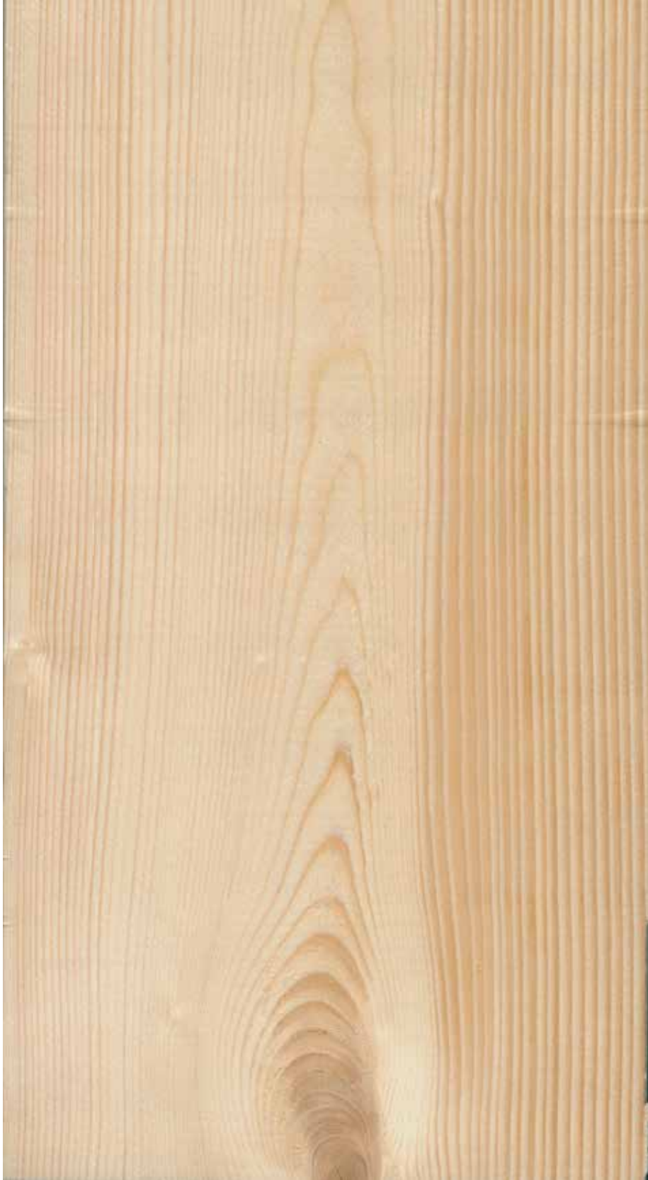
Figur 39. Kraftig tennar, planken vrakes.
