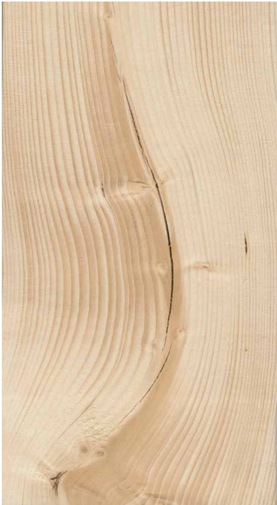
Figur 52. Stort toppbrudd, planken vrakes.
