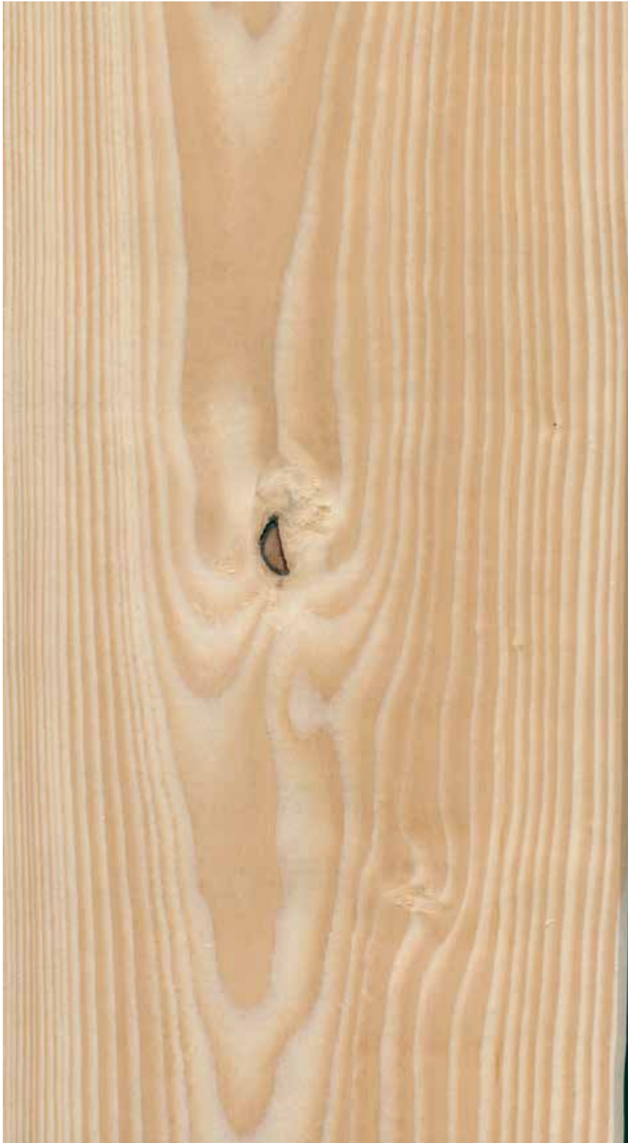
Figur 38. Kraftig tennar, planken vrakes.
