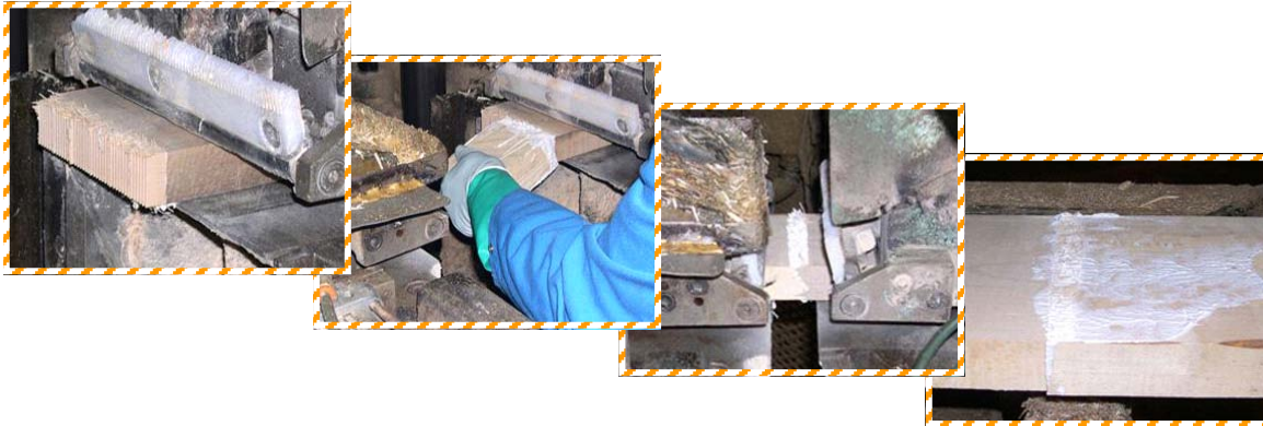
Figure 3.4. Finger jointing with EPI-adhesive: Process sequence.
