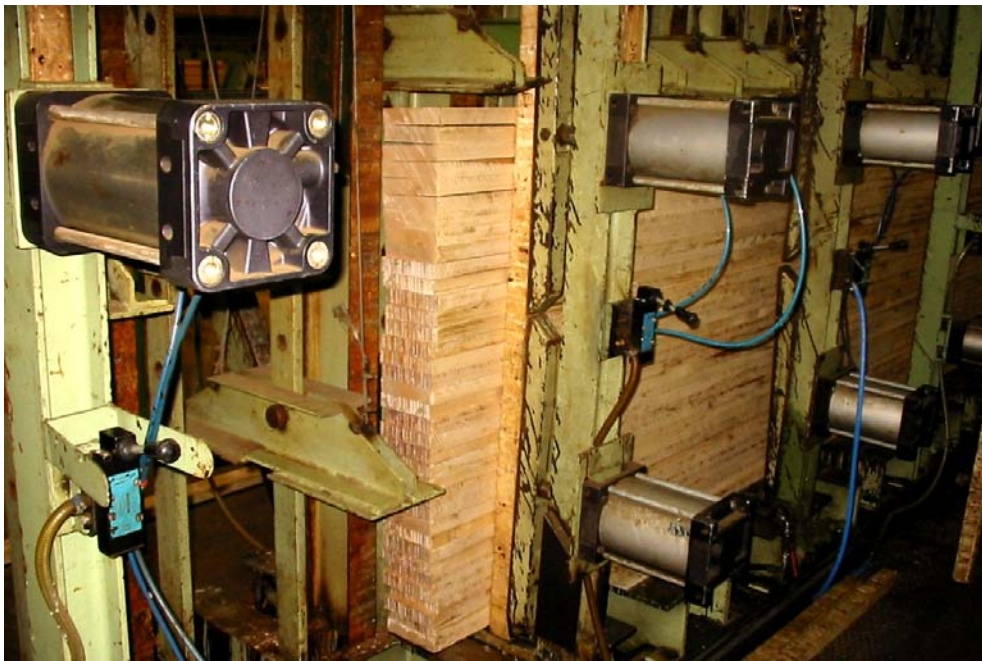
Figure 3.9. Beams in the press.
