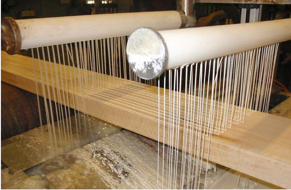
Figure 3.8. Applying of the adhesive.
