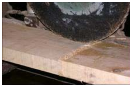
Figure 3.5. Finger joint right after pressing: MUF.
