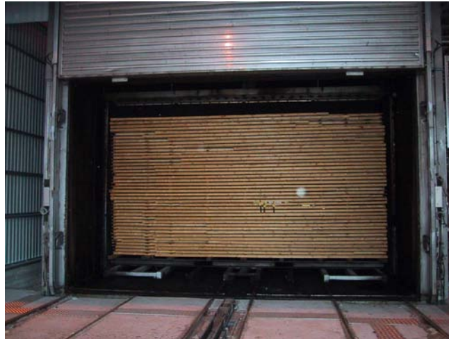
Figure 5.12. Timber in the Thermowood plant after drying at 120 °C at Stora Enso Timber, Kotka Sawmill.
