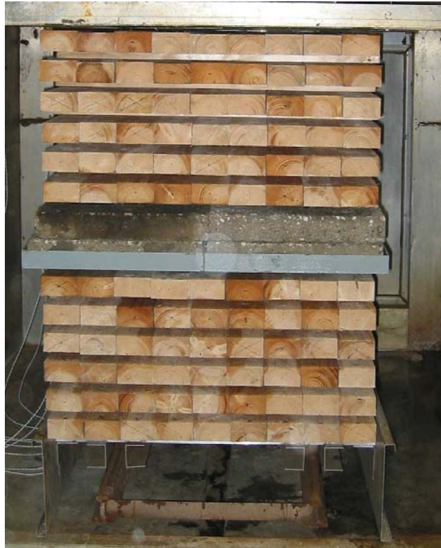
Figure 4.3. Front view of experimental stack, lower part loaded with 500 kg/m 2 , upper part unloaded.
