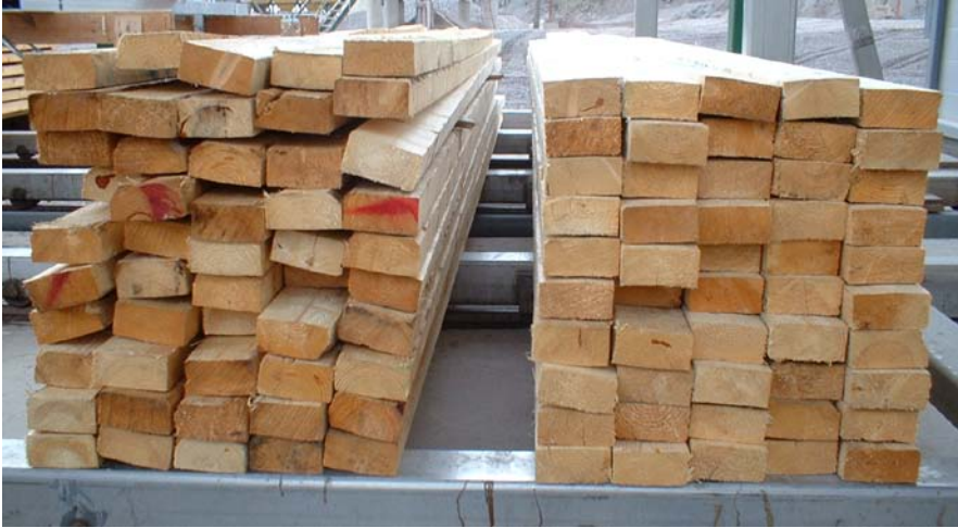
Figure 2.26. Loaded and unloaded battens after drying.
