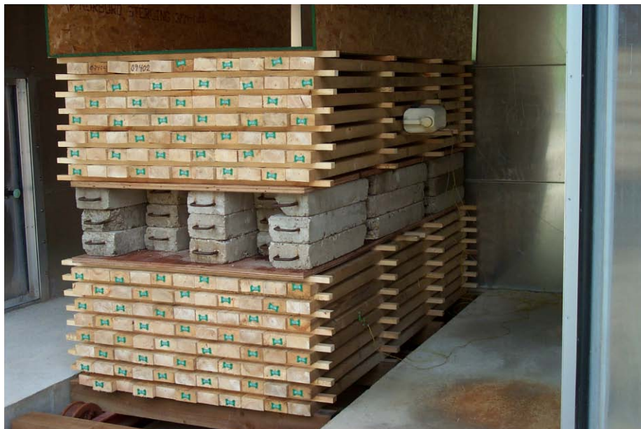
Figure 3.2. Front view of kiln load, lower part loaded with 480 kg/m 2 , upper section unloaded.
