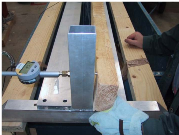
Figure 5.9. Jig for measuring deformations. Determination of twist.
