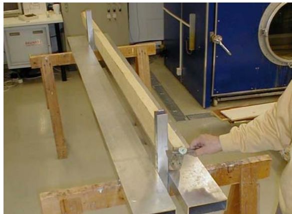
Figure 2.18. Test jig for the industrial tests.
