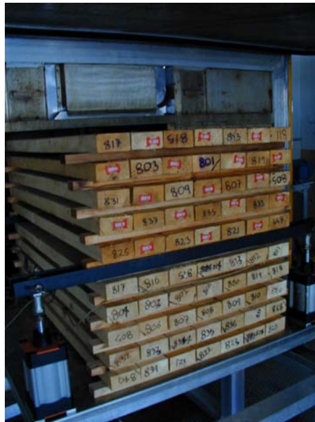
Figure 5.2. Drying charge in laboratory kiln. The bottom layer of timber is top loaded with aid of pneumatic cylinders. Species shown is Sitka spruce timber from UK.
