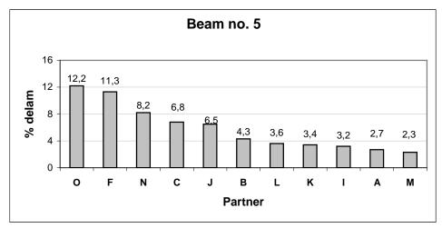
Figure 5.5Mean delamination for beam 5<br/>(long closed assembly time, 55 min)
