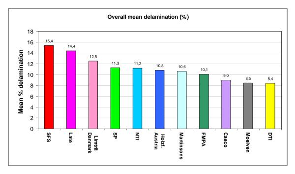
**Figure 7.7** Ranking for each partner and all beams, from the highest delamination (on the left side) to the lowest delamination (on the right side).
