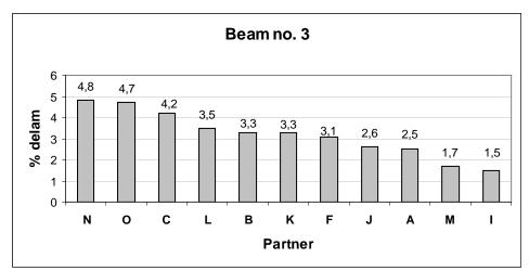
Figure 5.3Mean delamination for beam 3 (low glue spread)
