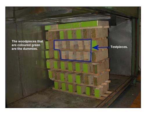
Photo 2: Wet samples should be placed in the middle of the sample pile. Samples consisting of dry dummies and wet samples should fill out the whole of the drying chamber's cross-section. Samples shall always be placed above each other and stand in a row, so that a corridor of 5 cm between samples is present. The air speed shall be measured in the middle of the pile in between the samples, with a closed chamber door."
