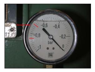
Photo 1: With this meter, the vacuum to be drawn shall lie between -0,70 and -0,85 bar (0 is atmospheric pressure, -1 is absolute vacuum).
