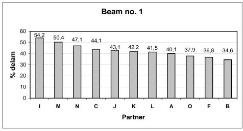
Figure 7.1Mean delamination for beam 1<br/>(very long assembly time, 80 min)
