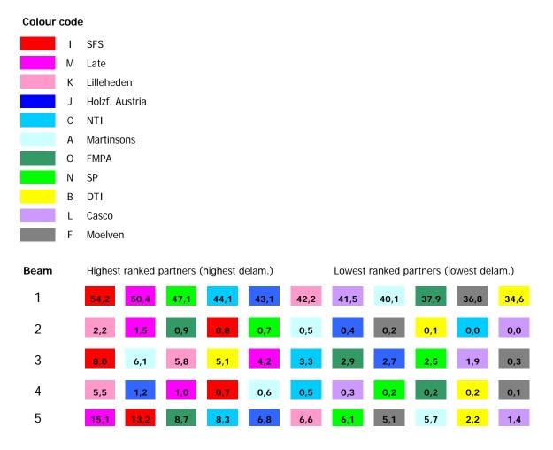
**Figure 7.6** Ranking for each partner and each beam, from the highest delamination (on the left side) to the lowest delamination (on the right side).
