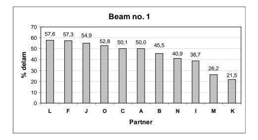
Figure 5.1Mean delamination for beam 1<br/>(very long closed assembly time, 80 min)
