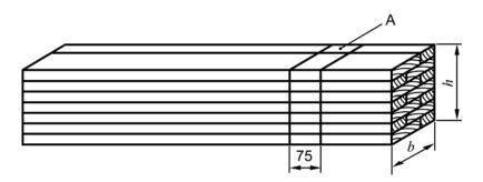
**Figure 1 - Test piece cut from a glulam member** Key: A Test piece Dimensions in millimeters
