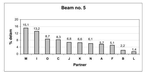
Figure 7.5Mean delamination for beam 5<br/>(long assembly time, 55 min)
