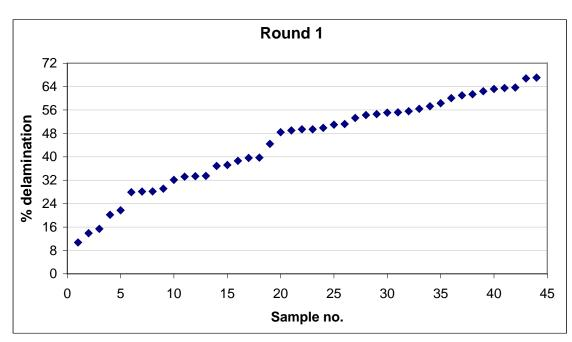
Beam 1 - 80 min. closed assembly time All obtained values are ranked from the lowest to the highest
