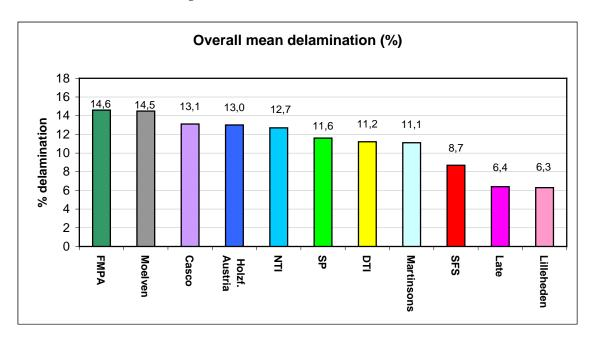
**Figure 5.7** Ranking for each partner and all beams, from the highest delamination (on the left side) to the lowest delamination (on the right side).
