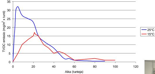
VOC emissions from painted surface in function of time (15 and 25°C) (water-based acrylic paint 10,2g/sample, loading factor 0,8m<sup>2</sup>/m<sup>3</sup>, air exchange 1.2 h<sup>-1</sup>. *Haghihat and Bellis, Building and Environment, Vol 33, 1998*)
